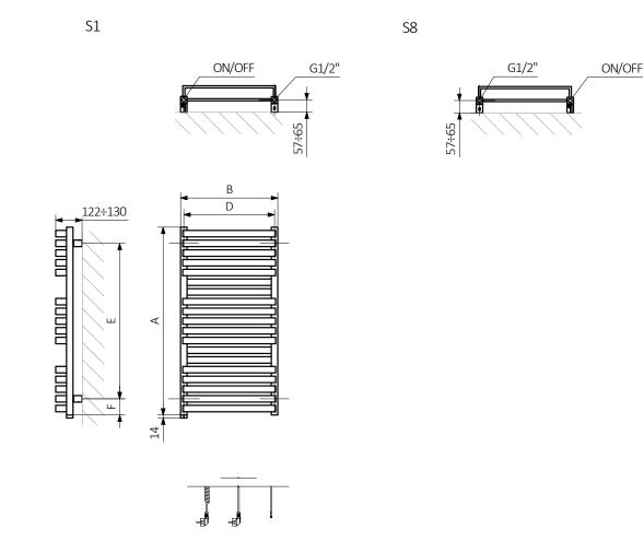
A - Height B - Width C1-C5 - Distance between pipe centres D - Horizontal distance between mounting bracket centres E – Vertical distance between mounting brackets F – Distance between a mounting bracket and the bottom of the radiator
